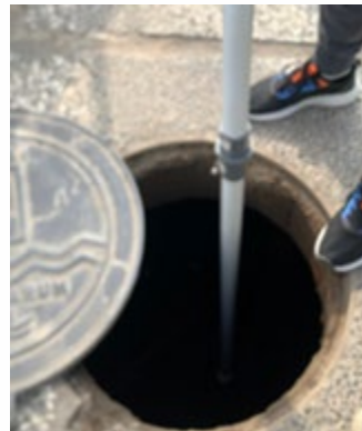
Take the sludge sample with DIY Sludge Sampler (pipe and foot valve)
