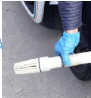
Take the sludge sample with DIY Sludge Sampler (pipe and foot valve)
