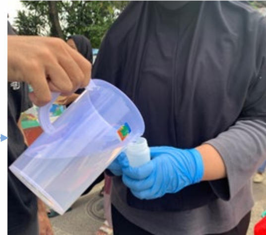
Put wastewater sample into plastic & glass bottles
